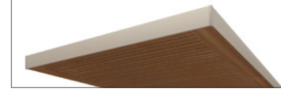
Aluminium roof frame + Wood-laminate ceiling
